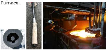
A solution based on image processing for LF slag viscosity estimation was developed and field validated.
